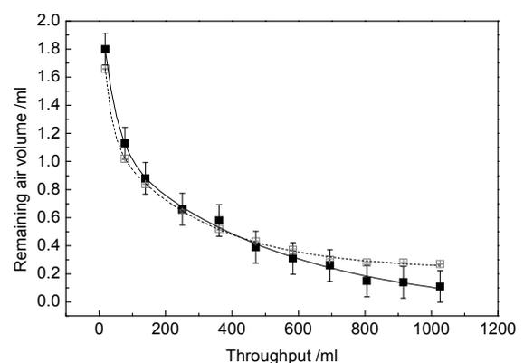
Figure 2 Verification of remaining air measuring method. At 20kPaG static pressure, using IPA, with pump dispense rate of 1ml / 2sec. □: Calculated by dispensing liquid weight, standard deviation is expressed by size of data point marker (open box). ■: Calculated by measured filter weight, error bars express standard deviation.
