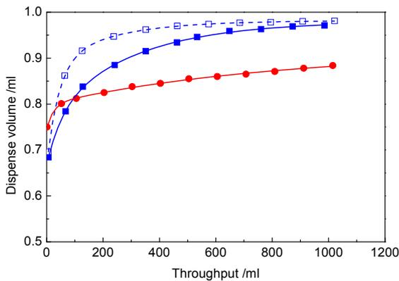
Figure 3 Dispense volume comparison among filter start up methods: ● Tubephragm pump driven method, ■ Static pressure driven method-1 (50 kPaG), □ Static pressure driven method-2 (100 kPaG).
