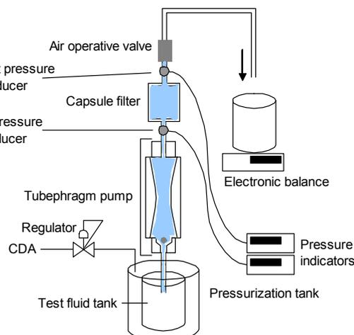
Figure 1 Test stand employed for remaining air measurement in capsule filter.
