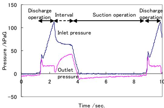
Figure 4 Pressure change during tubephragm pump operation.
